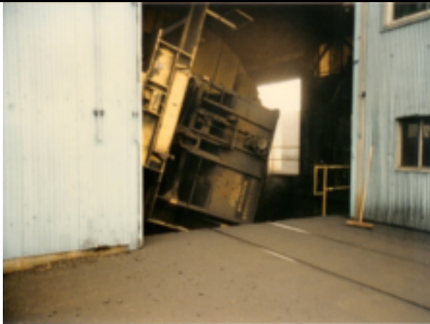
1997 Club trip to DP&L Indian River Power Plant. Rotary dump emptying a coal hopper
