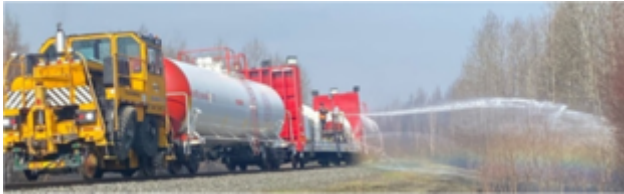
Canadian National has turned a flatcar, two tank cars, and a track maintenance vehicle into a firefighting train, dubbed Poseidon , fighting Alberta wildfires (Photo by CN)
