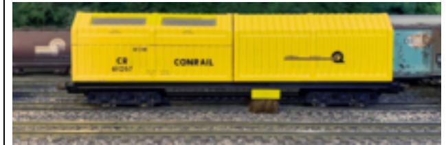
A vacuum car like this repainted HO scale Roco model can help keep dust under control on your right-of-way. (Dave Abeles photo)
