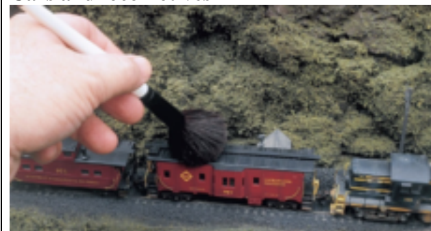
A soft, dry brush, like this one made for dusting camera lenses, works well to take dust off model structures and rolling stock. (Lionel Strang photo)
